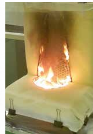
Seat fire test at CREPIM under EN 45545
